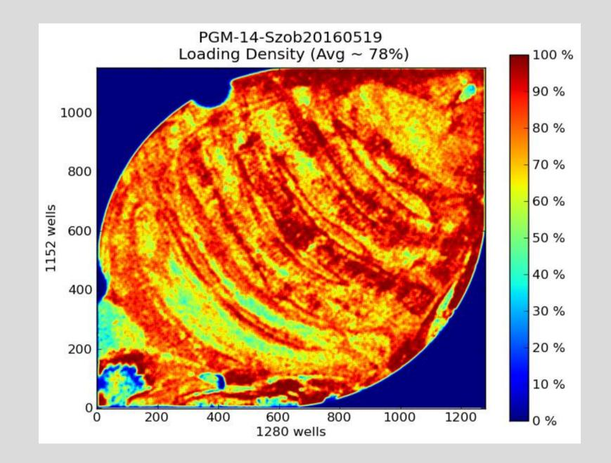
Loading density of the ION 314 Chip
